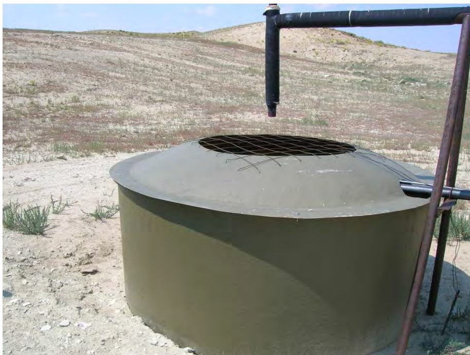
Figure 8. Dehydrator tank with a partially-covered top.
