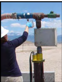
Left to right: sampling with a collection valve in place; when no valve is in place; and with bailers when no pump is in place.
